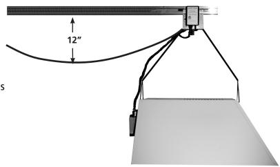
restriction. We recommend that there be at least 12 inches distance from the bottom of the rail to the center of the power cords arc when the cord's are fully extended and fasten both cords to the bottom of the Drive Motor. You can fasten to either of the two holes or the eye screw described earlier. Please do not fasten to the Motors Wires.
